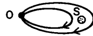
Fig. 4. Aharonov-Bohm experiment. S is a solenoid with magnetic flux perpendicular to plane of paper.
