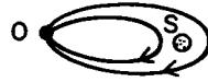
Fig. 4. Aharonov-Bohm experiment. S is a solenoid with magnetic flux perpendicular to plane of paper.
