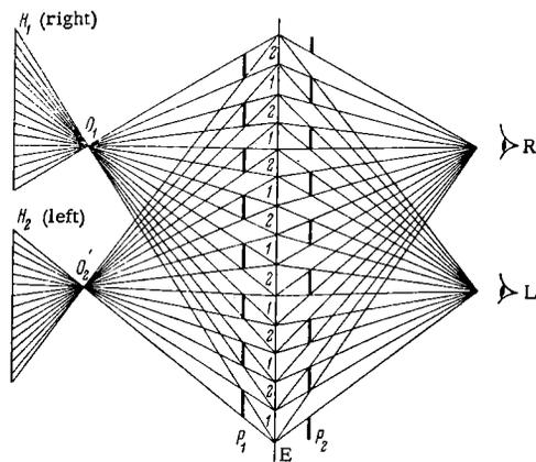
Fig. 1. Replacement of stereoscope by a line pattern screen:  $O_1, O_2$  are projection lenses,  $H_1$  and  $H_2$  are the two stereoscopic negatives,  $P_1$  and  $P_2$  are identical line pattern screens,  $E$  is a screen or a photographic film,  $L$  and  $R$  are the eyes of the viewer, 1 and 2 are alternating strips of the left and right images.
