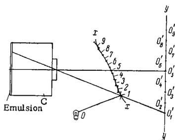
Fig. 4. Gramont and Planovern integral photographs: C is the camera; O is the subject; 1-9 are flat mirrors located on the curve XX in such a way that the subject images  $O_1'$ - $O_9'$  are located on the straight line YY, perpendicular to the axis of the camera C. The optical model is reconstituted at the site of the subject by projecting the positive through the same system of camera and mirrors.
