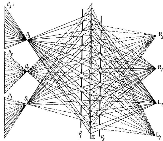
Fig. 2. Principles of a parallax panoramagram:  $H_1-H_3$  are negatives photographed in the camera with several lenses arranged in a row:  $O_1-O_3$  are projection lenses;  $P_1, P_2$  are identical line pattern screens;  $E$  is a screen or a photographic plate;  $L_1$  and  $R_1, L_2$  and  $R_2$  are the positions occupied by the eyes of the viewer while shifting perpendicularly to the line direction on the pattern; 1, 2, 3, are alternating image strips.
